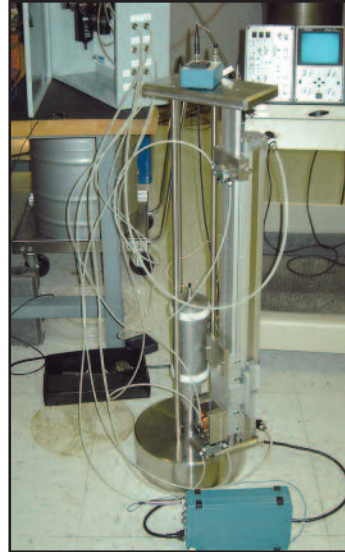
High Pressure Hydraulic Impulse Calibration (to 100,000 psi)
