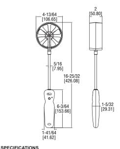
Service: Clean air. Temperature Limits: Process: -4 to 140°F (-20 to 60°C); Ambient: 5 to 125°F (-
