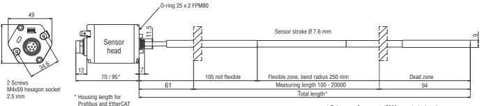
\* Tolerance +8 mm up to 7600 mm stroke length Tolerance +15 mm -5 mm > 7600 mm stroke length Tolerance of total length has no influence to the stroke length
