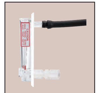
Model MMF connections. Connector at top, installed in panel, has retainer and flexible tubing in place. Connector at bottom shows alternative connection with metal or rigid plastic tubing, using a double compression nylon tube union (as Dwyer Part No. A-328).
