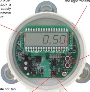
· Digital Push Button Zero and Span. Reduces calibration time significantly over other transmitters that utilize potentiometers. Lowers maintenance time and costs.
