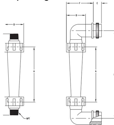
The Series LFM In-Line Flowmeter measures the flow of water and other compatible media. Models possess dual GPM and LPM scales. Various size ranges and connections are available to satisfy your application.
