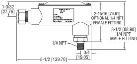
The Series 626 and 628 Pressure Transmitters converts a single positive pressure into a standard 4-20 mA output signal. The Series 626 and 628 can be used to accurately measure compatible gases and liquids; Series 626 full scale accuracy is 0.25%; Series 628 full scale accuracy is 1.0% (see specifications). Designed for industrial environments with a NEMA 4X (IP66) housing, this transmitter resists most effects of shock and vibration.
