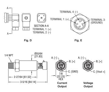
Fig. F: Packard Connection
