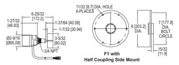
The **MODEL DBLM** Mini-Bin Dry Bulk Level Monitors provides reliable level sensing for dry bulk solids where mounting space is limited. Model DBLM Mini-Bin operates by using a 1 rpm synchronous motor to rotate a four vane, plastic paddle, and when material surrounds paddle and impedes rotation, the motor is de-energized and triggers a SPDT snap switch. Mount the Mini-Bin with optional 1-1/4" to 3/4" reducer to replace standard size units.
