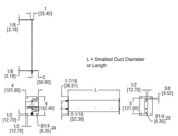
The SERIES DAFM Duct Air Flow Measuring Probe uses evenly distributed total and static pressure measuring points to deliver an accurate measurement of velocity pressure in a duct.
